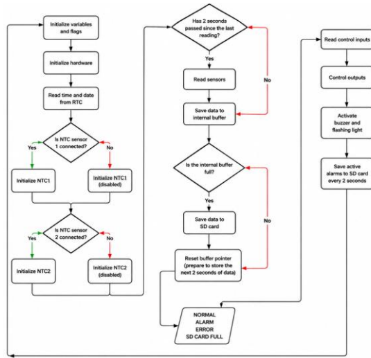
Fig. 6. Irrigation System Flowchart.
