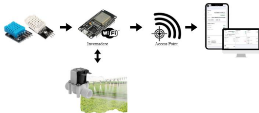
Fig. 7. Data Communication Diagram and IoT Interface
