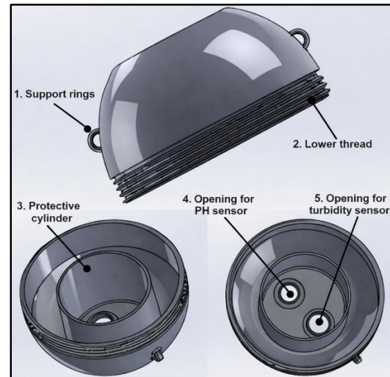
Fig. 5. Lower cover design (Sensor Node). Source: own elaboration.
