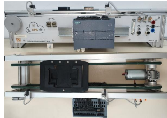
Fig. 3. Lucas-Nuelle Cyber-physical conveyor system with PLC.
