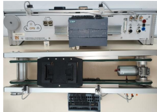
Fig. 3. Lucas-Nuelle Cyber-physical conveyor system with PLC.
