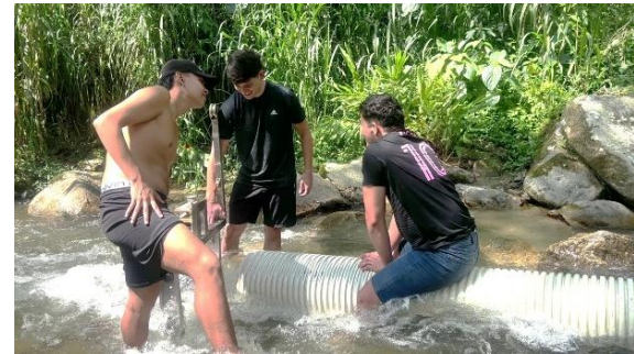
Fig. 4. Tests with PVC pipe channeling for flow stabilization. Fuente: Source: own elaboration.
