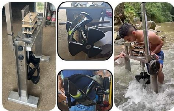
Fig. 3. Manufactured module, 3D-printed rotor, and free-flow testing (without channeling) Source: own elaboration.
