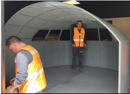
Fig. 11 C-130 cab assembly Source: Authors.
