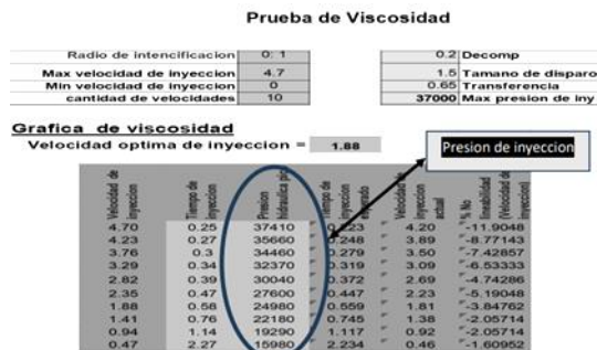
Fig. 2. Injection pressure within the viscosity curve test. Source: own elaboration
