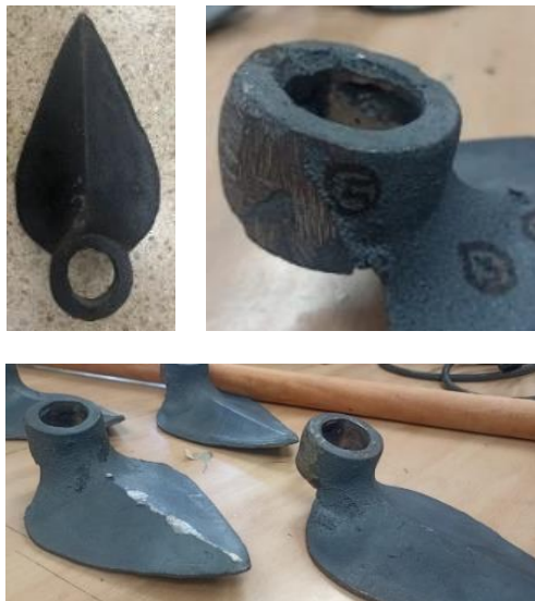
Fig. 10. Final casting in ASTM A536 cast iron (authors).
