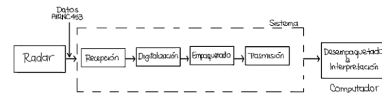
Fig. 3. General communication architecture of the ART-2000 weather radar.
