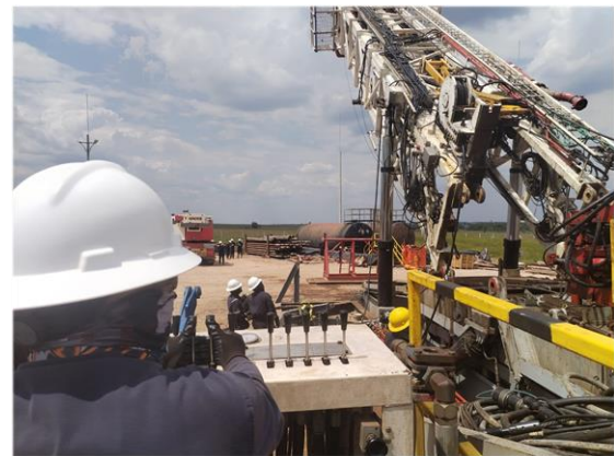
Fig. 1. Operator's perspective at the mast hoisting controls – limited visibility for transverse leveling.
