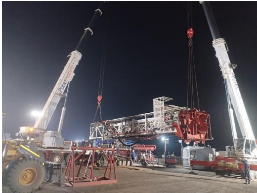
Fig. 6. Mast hoisting using telescopic cranes — procedure used to obtain the weight of the NOV Rapid Rig 13 mast. Source: Authors.
