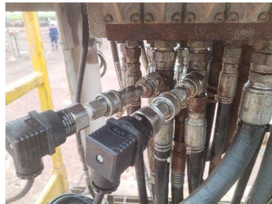
Fig. 5. Pressure sensors installed at the outlet of the 'mast raising' console valves. Source: Authors.
