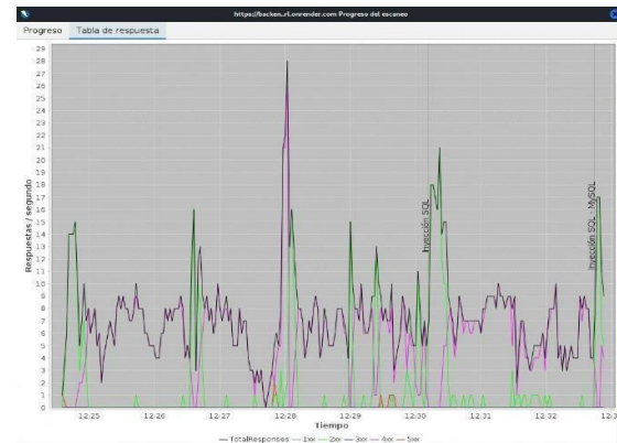
Fig. 11. Response graph - spidering attack. Source: Owasp-zap.
