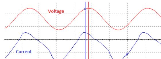
*Fig. 1. Voltage and current characteristics at the input of a single-phase rectifier with an inductive load and no PF correction. Source: own elaboration.*
