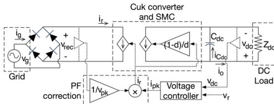
Fig. 3. Rectifier considering the action of the SMC and the PF correction strategy.
