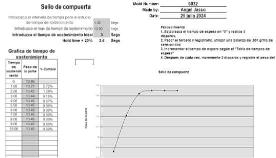
Fig. 3. Damper seal test. Source: own elaboration
