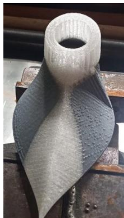
Figure 5. Prototype through 3D printing with corrections in the eyelet dimensions (authors).
