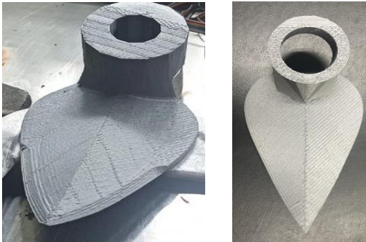
Fig. 4. Initial prototypes through 3D printing (authors).
