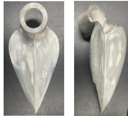
Fig. 9. Aluminum casting prototype, with 3D printed mold (authors).
