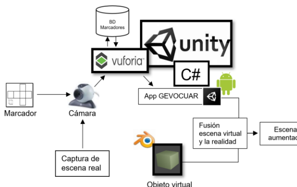
Fig. 5. Technological architecture of the prototype
