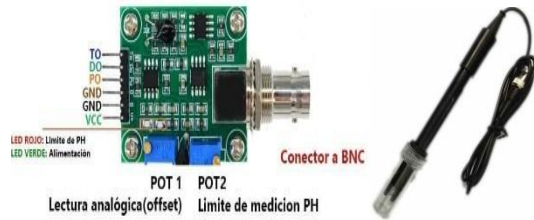
Fig. 5. Signal conditioning module and pH electrode.
