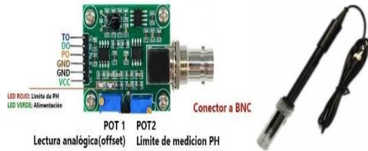
Fig. 5. Signal conditioning module and pH electrode.
