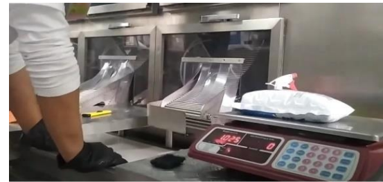
Fig. 21. Measurement of weight of freshly packaged milk bag" Source: own elaboration.
