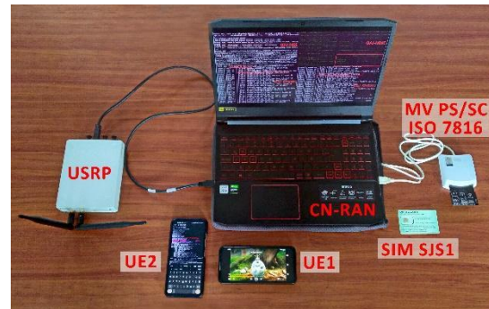
Fig. 8. Actual assembly of the CN and RAN. Source: Own elaboration.
