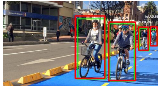
Fig. 4. Calculation of the Intersection over Union (IoU) for an image from the evaluation group. The green box indicates the ground truth region, while the red box indicates the detection region.
