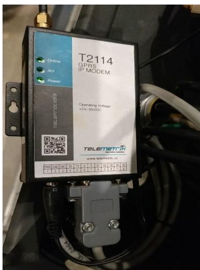
Fig. 6. Inverter communications system. Source: own elaboration.
