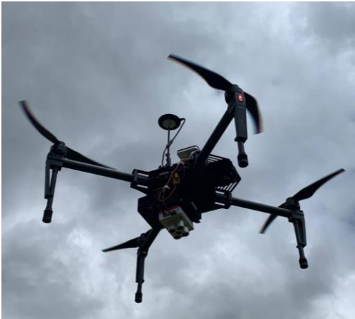
Fig. 2. Drone with a multispectral camera Source: own of the author.
