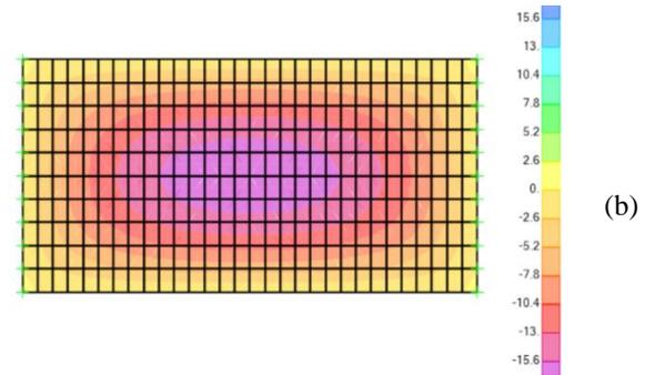
Figura 3. (a) Flexo-compresion behavior of 12x50x98cm solid plates. (b) Bending and shear behavior of 12x50x98cm solid plates.
