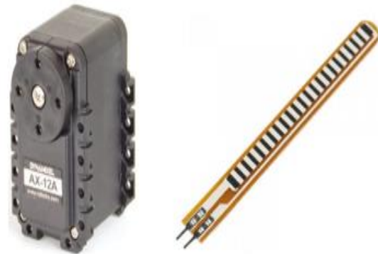
Fig. 4. Servomotor and flexo-sensor applied
