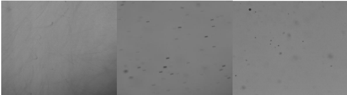
Fig. 2. Comparison of drop shadow images obtained from the same source with different shutter times: 1.6 ms (left), 0.16 ms (center), and 0.016 ms (right).
