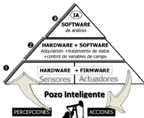
Fig. 1. Components of a smart well.
