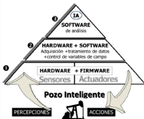
Fig. 1. Components of a smart well.
