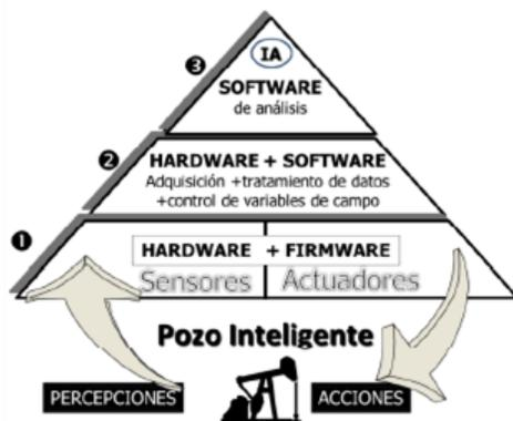
Fig. 1. Components of a smart well.
