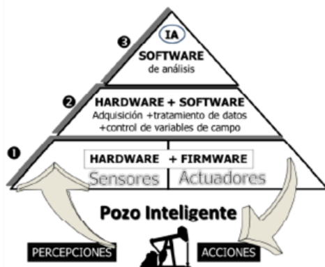
Fig. 1. Components of a smart well.
