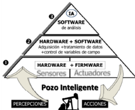
Fig. 1. Components of a smart well.
