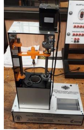
Fig. 3. Headspace Sampling (imagen propia)
