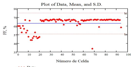
*Fig. 11 Graphic Representation of the Filling Factor Measurements with their Respective Mean Value and Errors*
