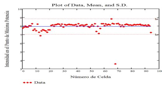
*Fig. 10 Graphic Representation of the Measurements of the Intensity at the Point of Maximum Power with its Respective Average Value and Errors*
