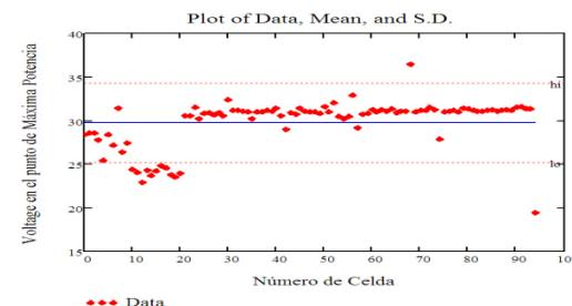
*Fig. 9 Graphic Representation of the Measurements of the Voltage at the Point of Maximum Power with its Respective Mean Value and Errors*
