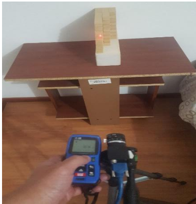
Fig. 10. Validation of depth with a digital laser distance meter
