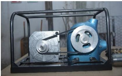
Figura 8. Micro turbina Pelton compacta
