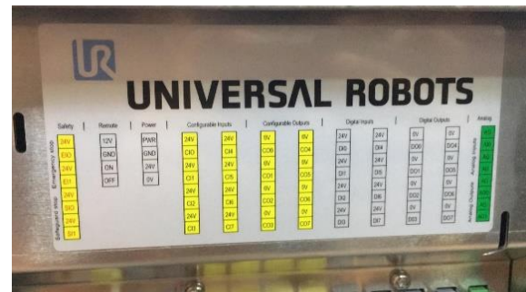
Fig 32. Diagram of the accessible terminals of the cobot controller
