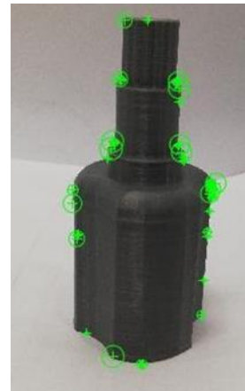
Fig 10. Surf characteristics of the piece to be handled
