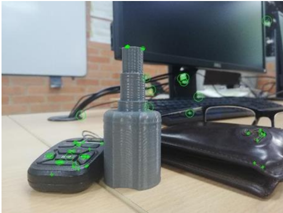
Fig 11. Surf features found in the validation photo.
