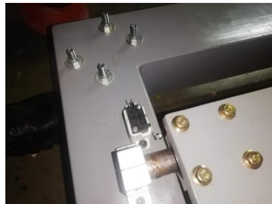
Fig 7. Base of the final stroke sensors
