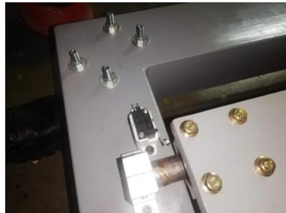
Fig 7. Base of the final stroke sensors
