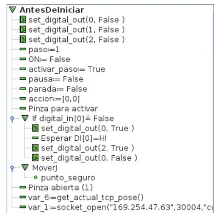
Fig 28. Initialization code on the robot
