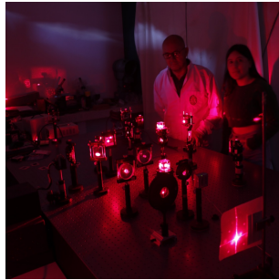
Figure 5: Experimental holographic setup for real-time recording and reconstruction. Source: Authors.
