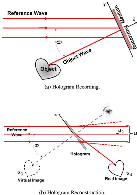
**Figure 3:** Schemes for Off-Axis hologram recording-reconstruction. Source: Authors.
