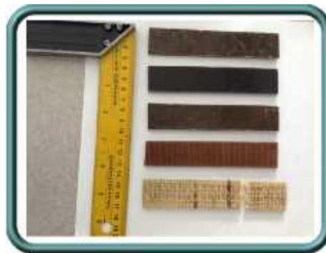
Figura 1. Sistemas bioepoxy-fibra.
